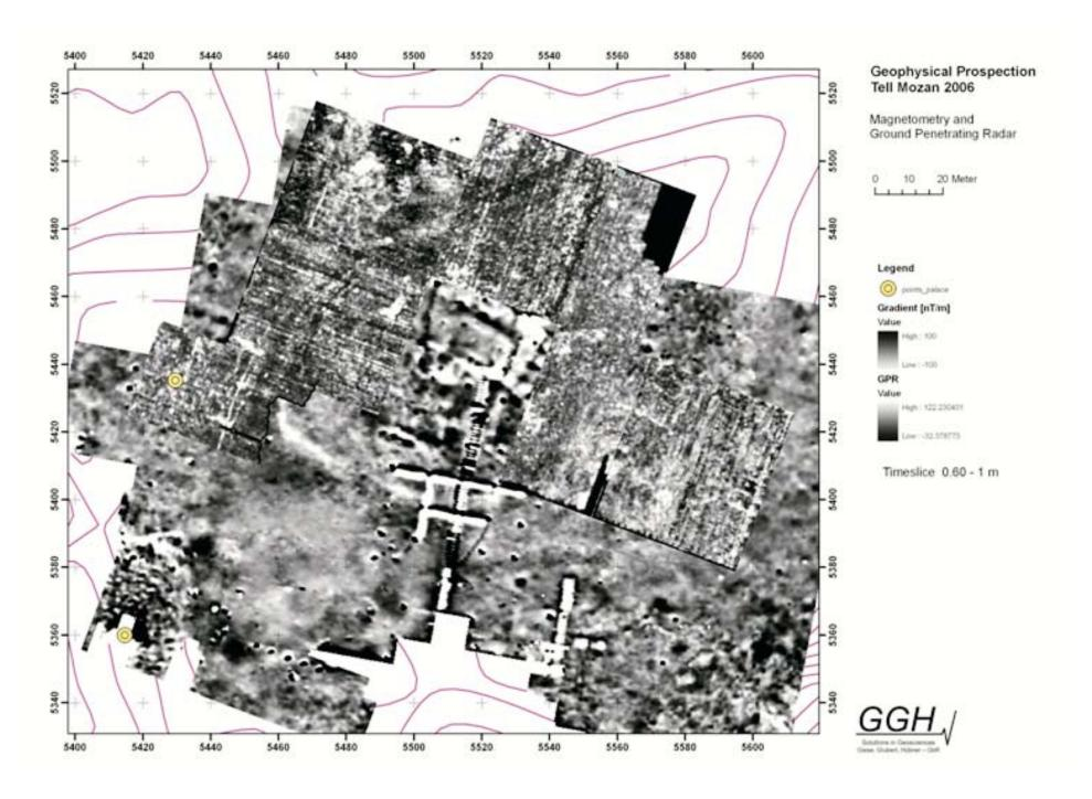
Fig. 41 Geo-physical survey: magneotmetry and ground-penetrating radar (overlaid)
